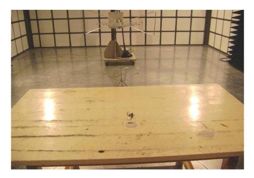
Radiation Emission Test View For 1GHz-25GHz
