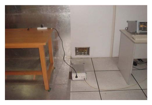
Radiation Emission Test View For 30MHz-1000MHz
