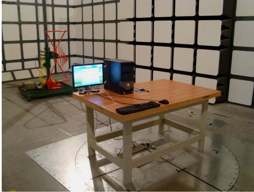
Below 1 GHz: Spurious Radiated Emissions - Front View (Transmitting mode)
