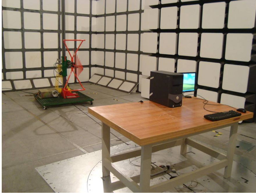
Below 1 GHz: Spurious Radiated Emissions - Front View (Charging mode)
