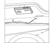
Attach the back of **BTK-810** to the fixed metal clip. The **BTK-810** must be placed in such way that its microphone is directed to the mouth of the user.
