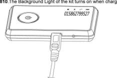
When the battery is full, the Background Light of the kit will turn off.The kit will be fully charged in approximately 2 to 4 hours.
