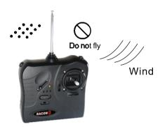
Extend the antenna to its full length. If the antenna is too short, the effective range of the radio waves will become shorter.
