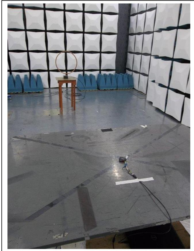
**Radiated Spurious Emissions, 30 MHz to 1000 MHz**
