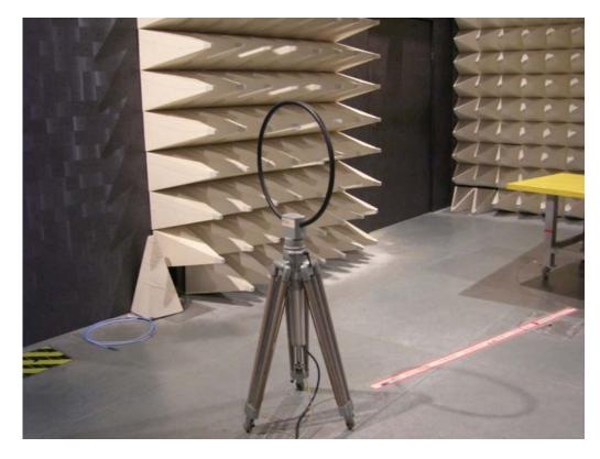
For radiated emissions 30MHz~1GHz
