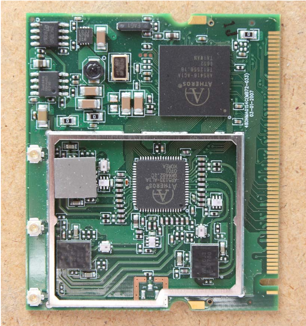
Transmitter Board without Cover – Front
