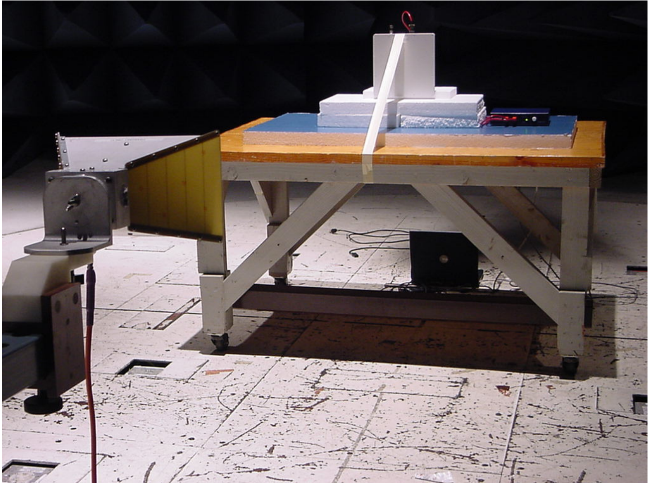
Photograph 4. Radiated Emission Spurious Test Setup
