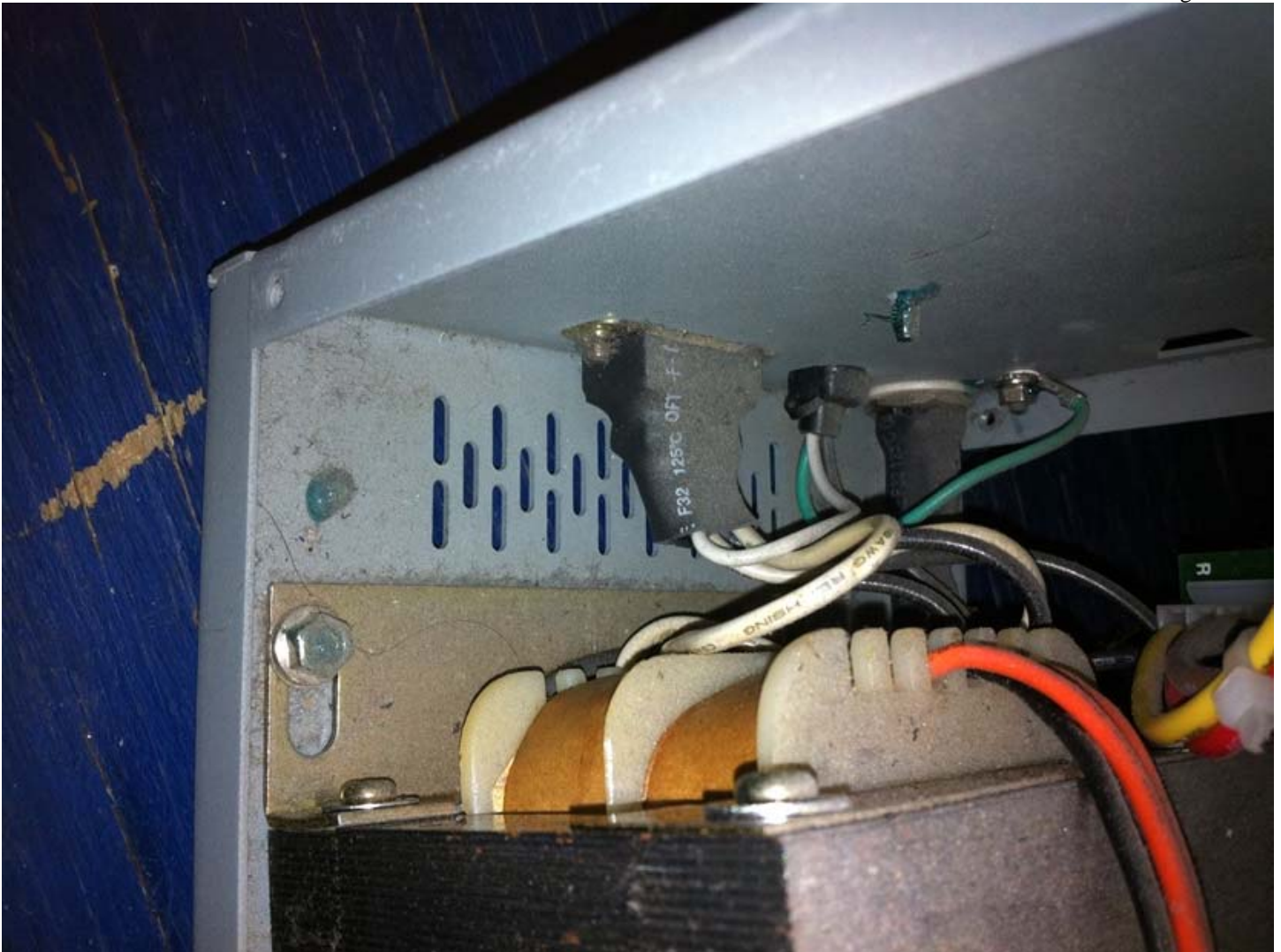
Inside View – Rear Panel – AC Voltage Range Switch Center, Mains Entry Point Visible (Green/White/Black Wires)
