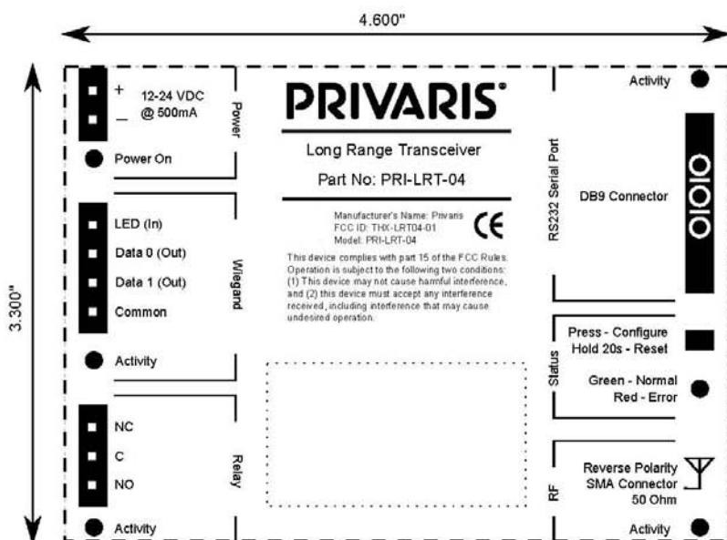
Sample Data for unused area above (Not Printed). The barcode contains the serial number, verbatim in Code 93.
