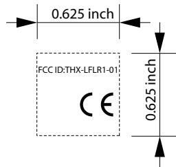
NOTE: Dashed line represents label cut lines (dimensions of cut label are 0.625 inch by 0.625 inch)
