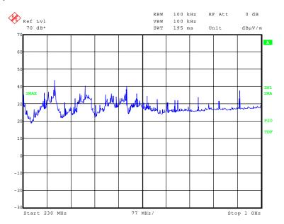
The following frequencies were found emission test outside and inside restricted bands during the preliminary radiated:
