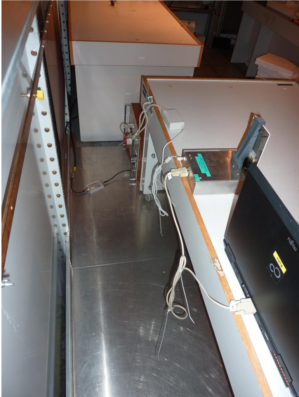
172416_25.jpg: SmartScan, test set-up shielded chamber
