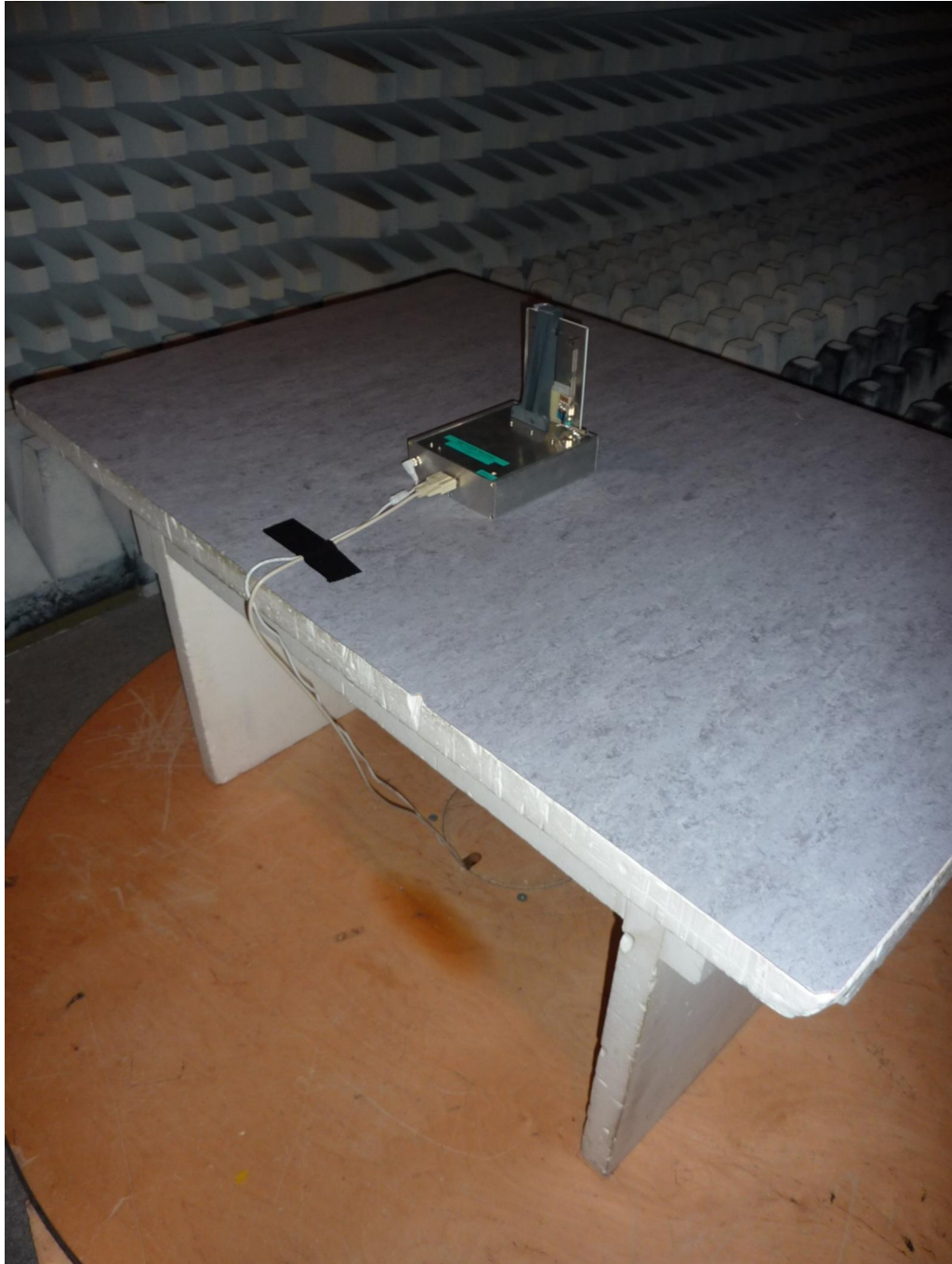
172416_6.jpg: SmartScan, test set-up fully anechoic chamber
