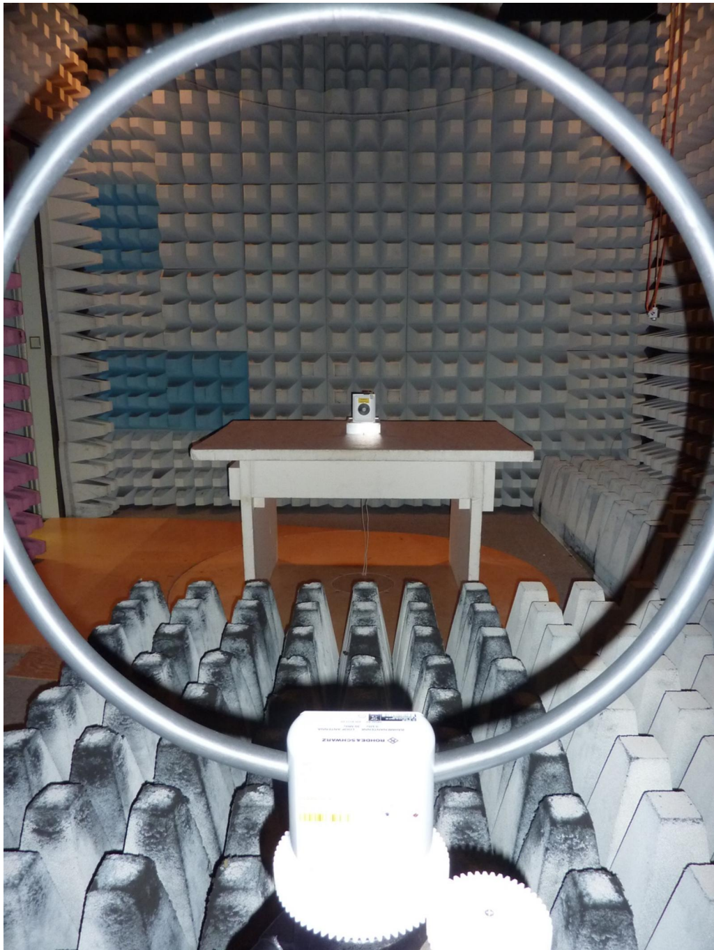
172416_8.jpg: SmartScan, test set-up fully anechoic chamber
