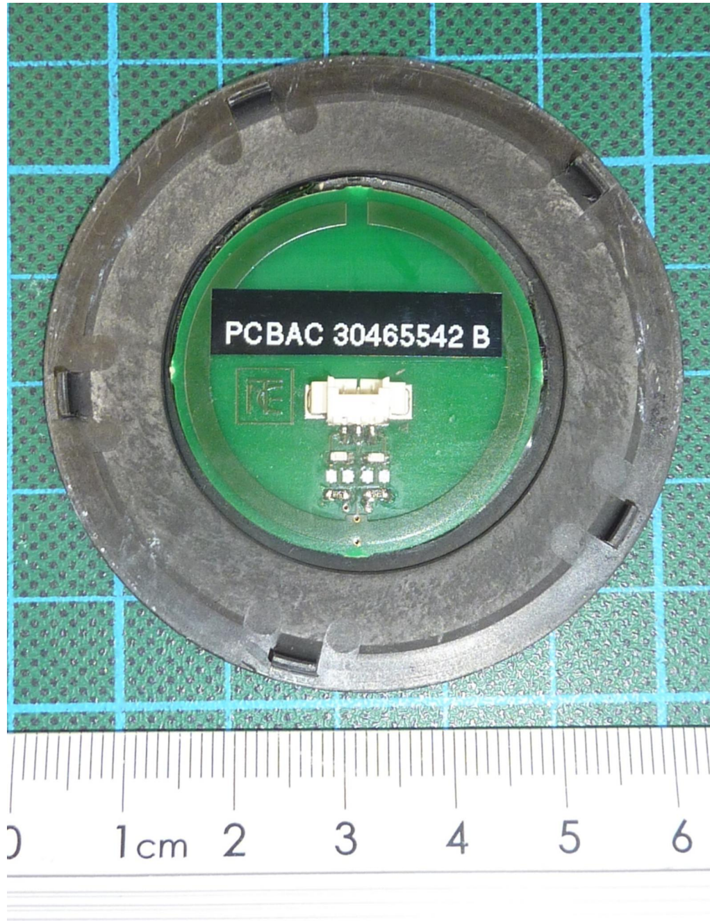
172416_o.jpg: SmartScan, antenna PCB
