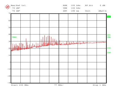
The following frequencies were found outside restricted bands during the preliminary radiated emission test:
