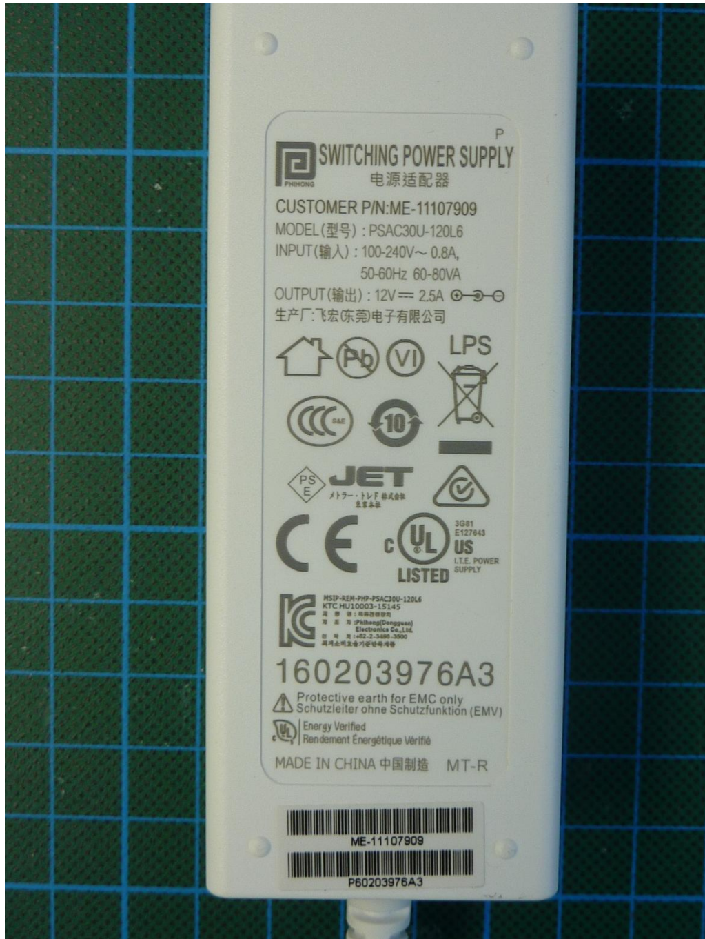
161000_1.jpg: SmartSample, type plate of dedicated AC/DC adaptor
