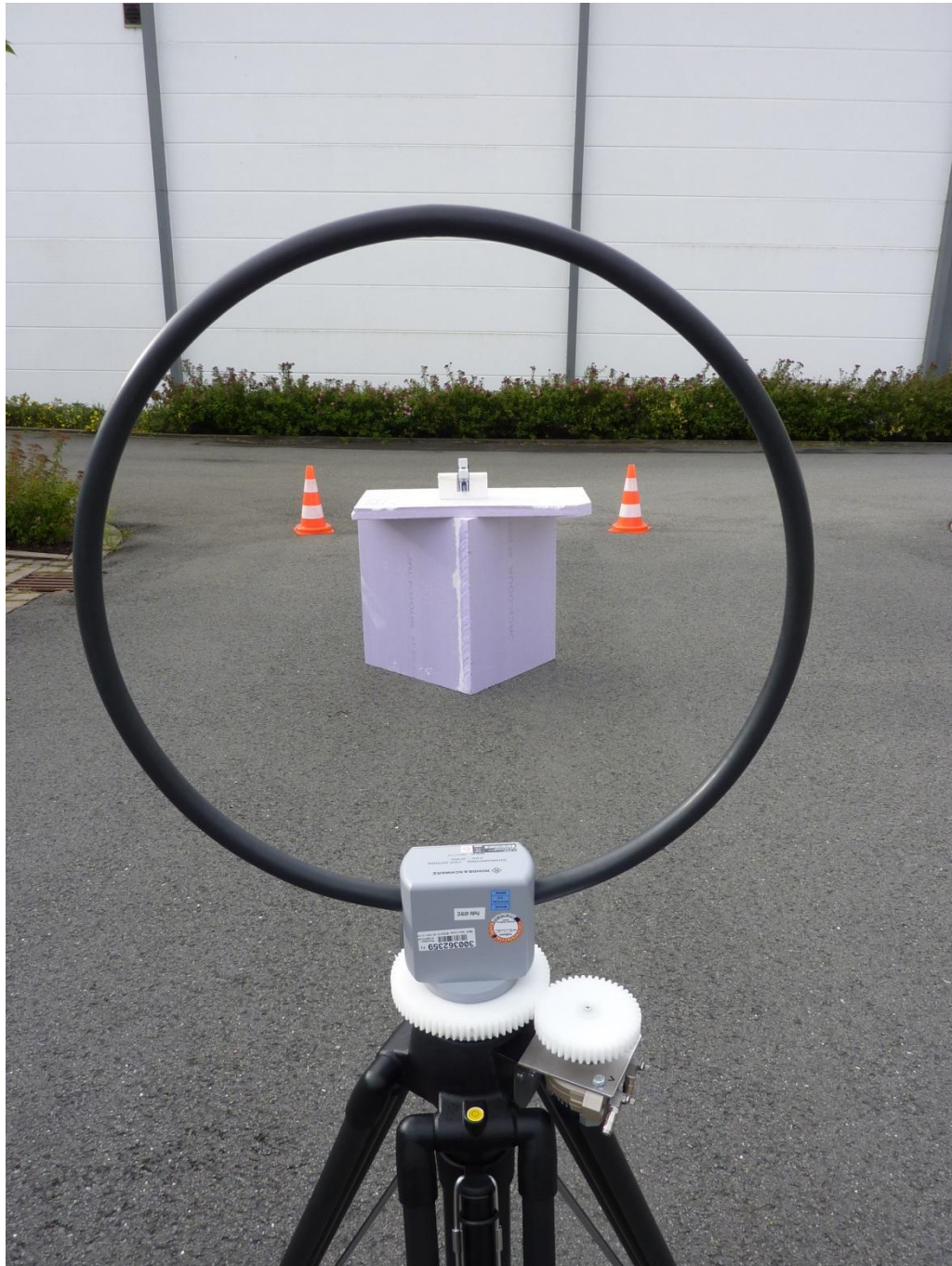
161007_1g.jpg: Quantos HPD, test setup outdoor test site
