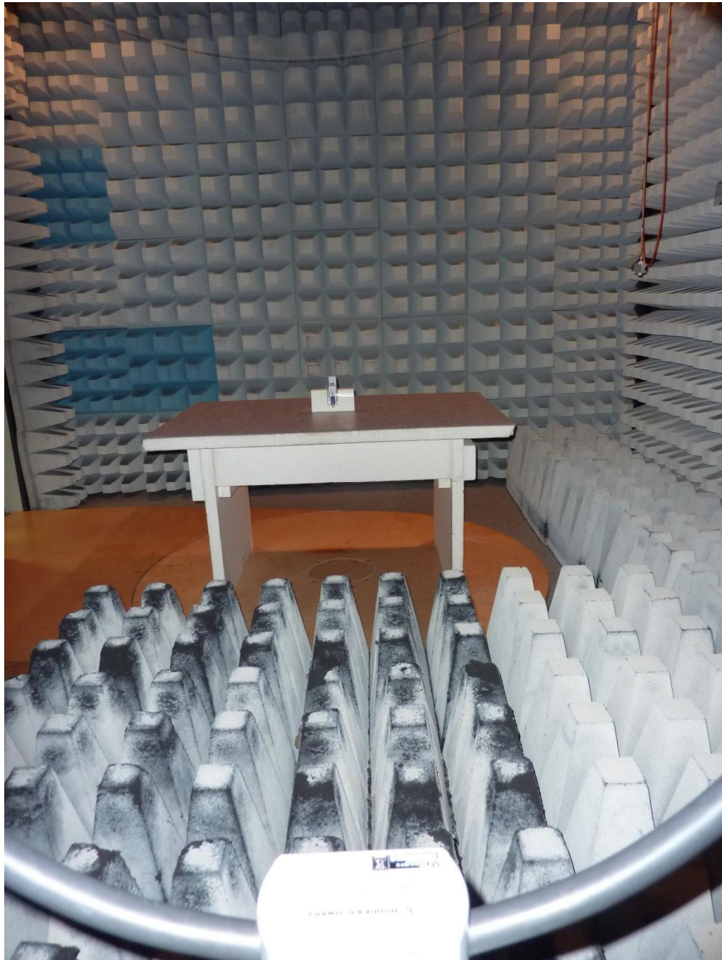
161007_1d.jpg: Quantos HPD, test setup fully anechoic chamber
