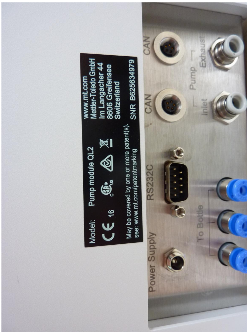
161006_13.jpg: Pump module QL2 (host), rear / type plate view
