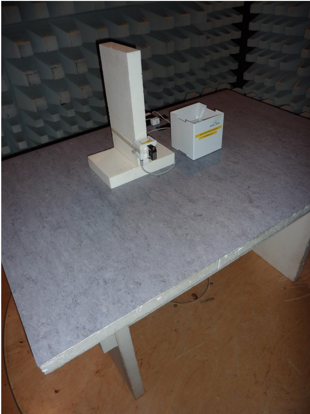
161006_1b.jpg: QLX45 Liquid Dosing Module, test setup fully anechoic chamber
