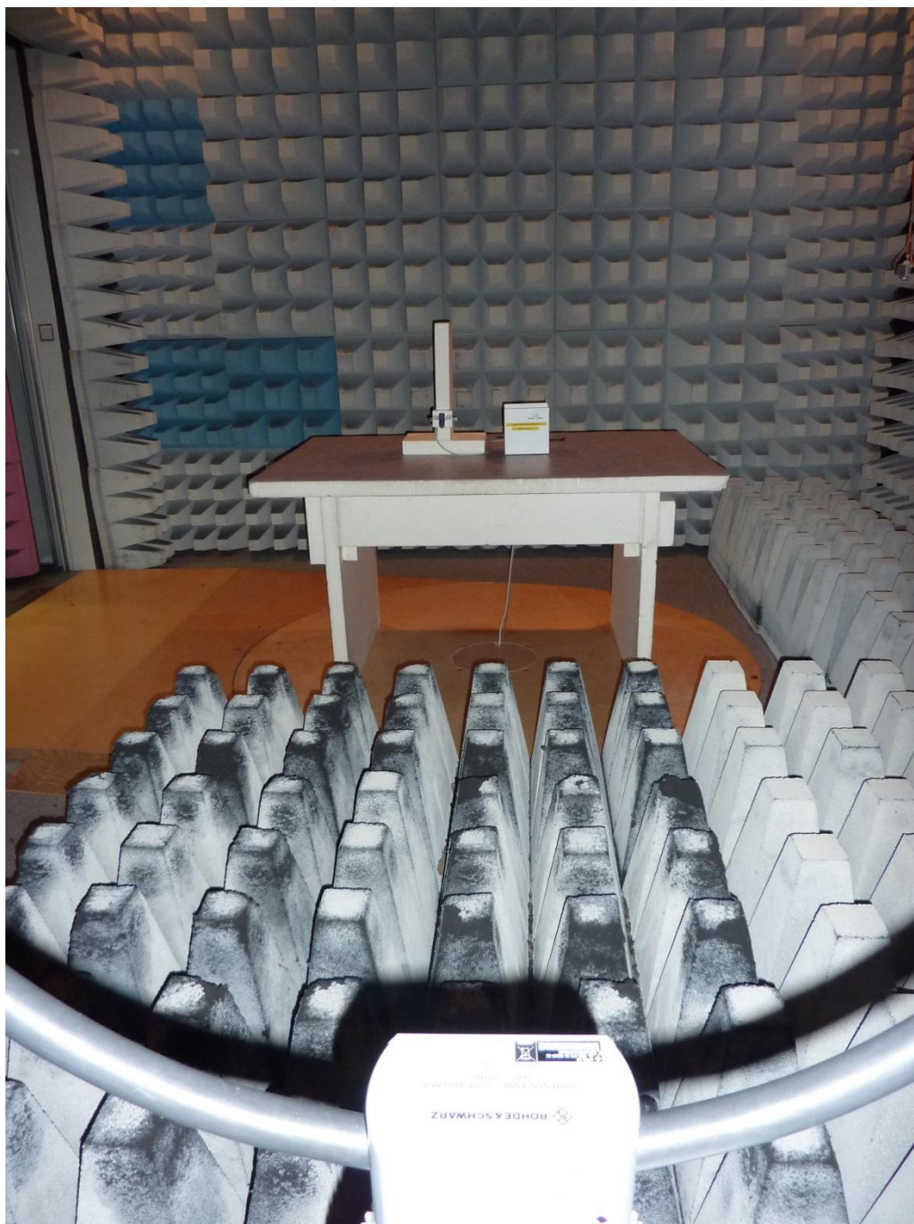
161006_1c.jpg: QLX45 Liquid Dosing Module, test setup fully anechoic chamber
