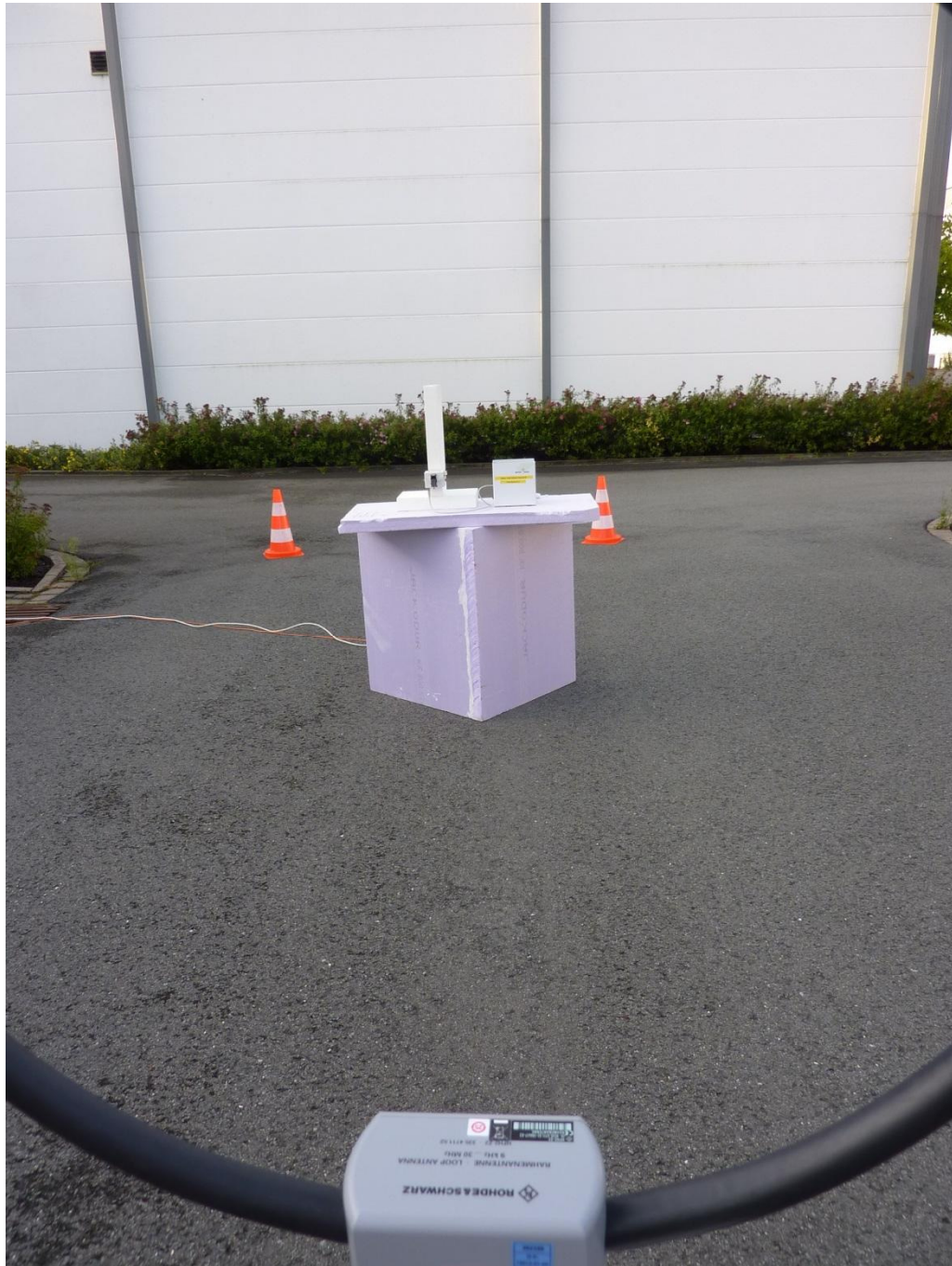
161006_1e.jpg: QLX45 Liquid Dosing Module, test setup outdoor test site
