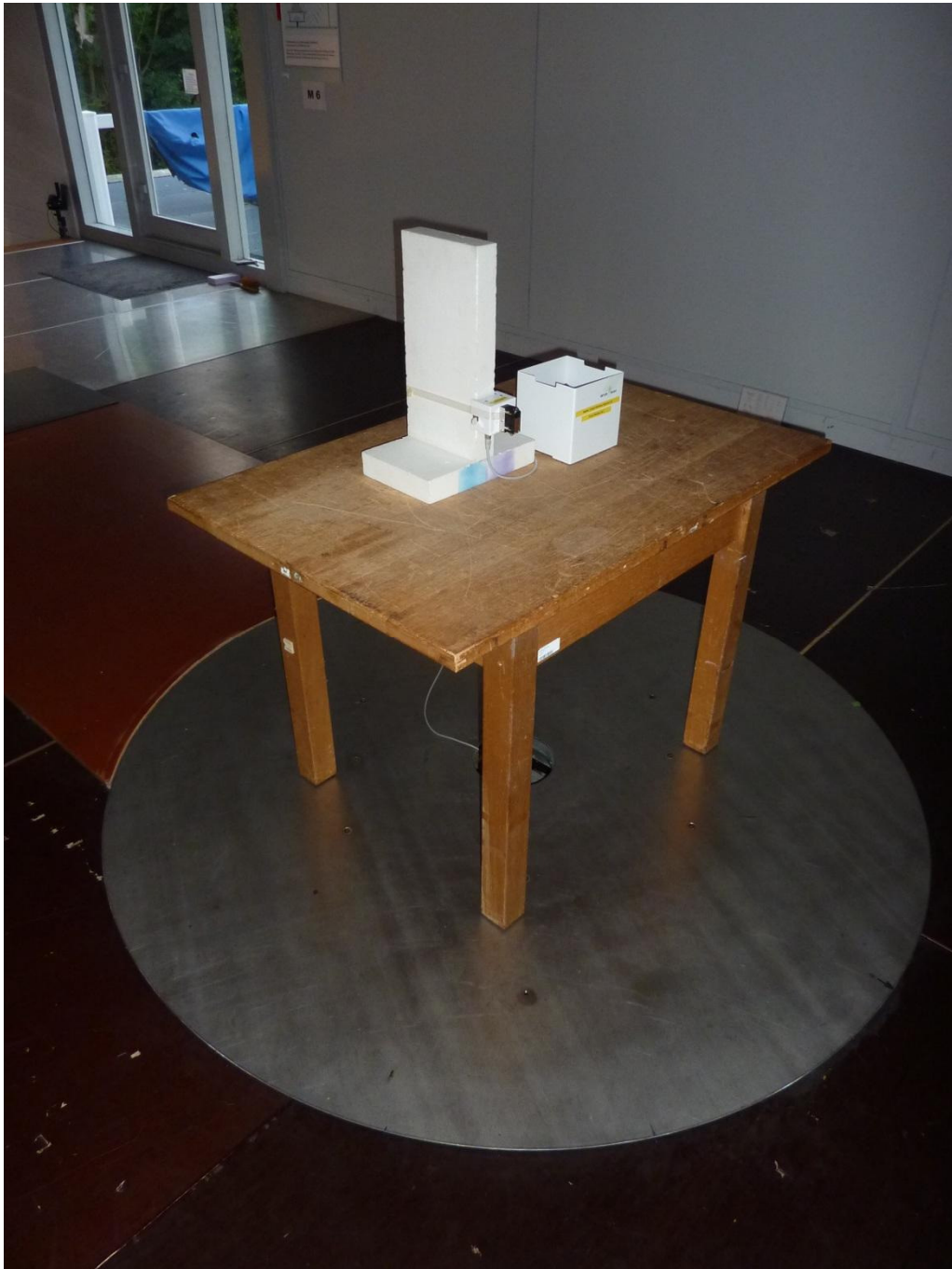
161006_1f.jpg: QLX45 Liquid Dosing Module, test setup open area test site
