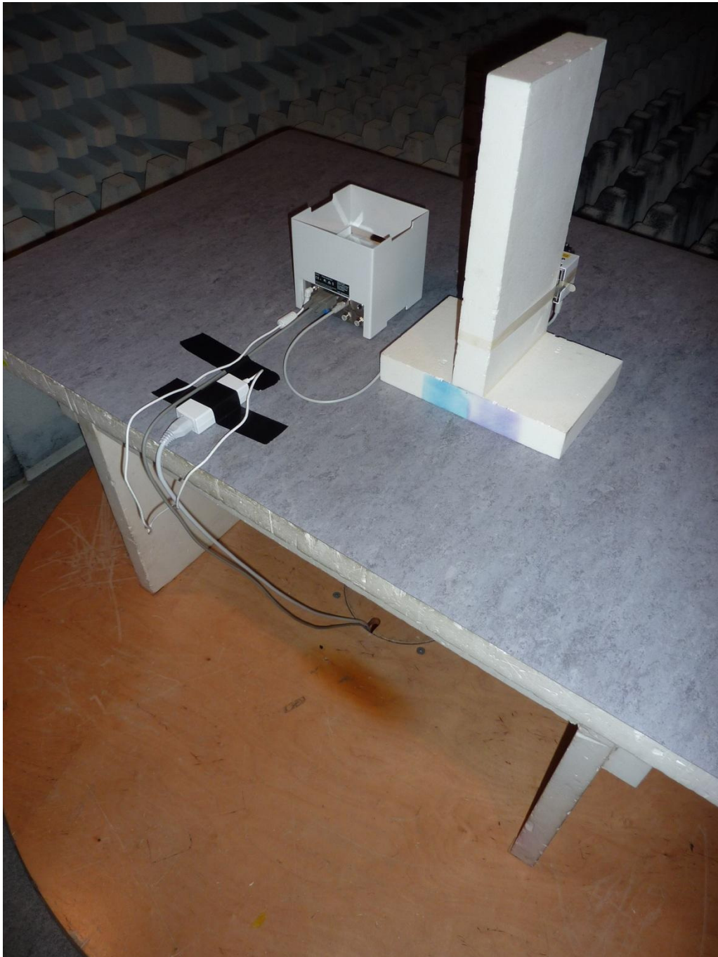
161006_1a.jpg: QLX45 Liquid Dosing Module, test setup fully anechoic chamber
