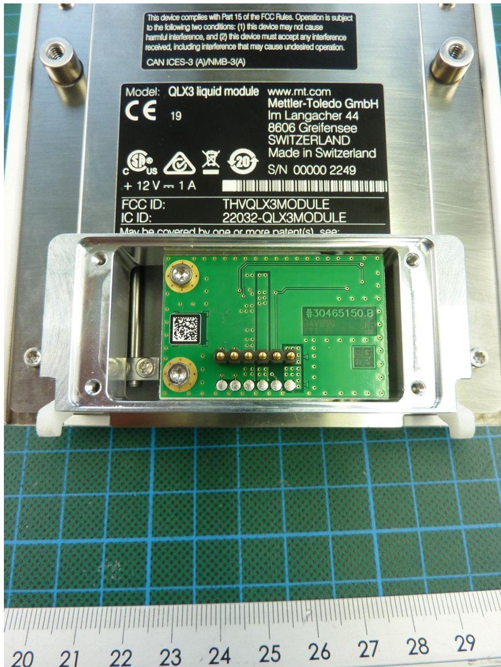
181223_13.jpg: QLX3 liquid module, internal view, rear cover opened
