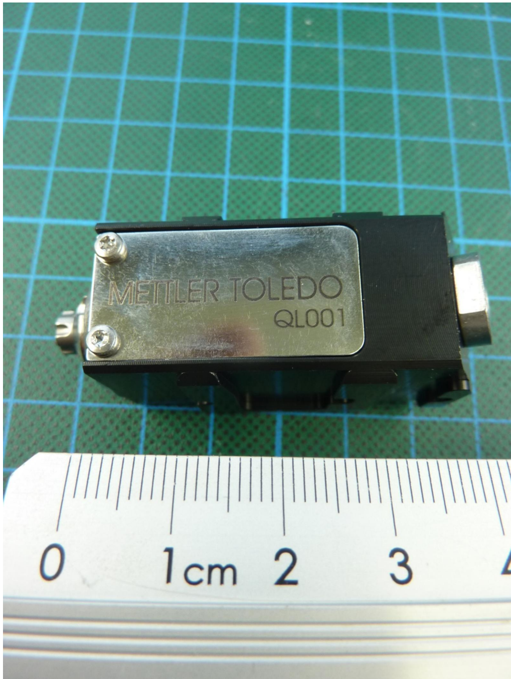
181223_18.jpg: Dosing head QL001 (with TAG), front view
