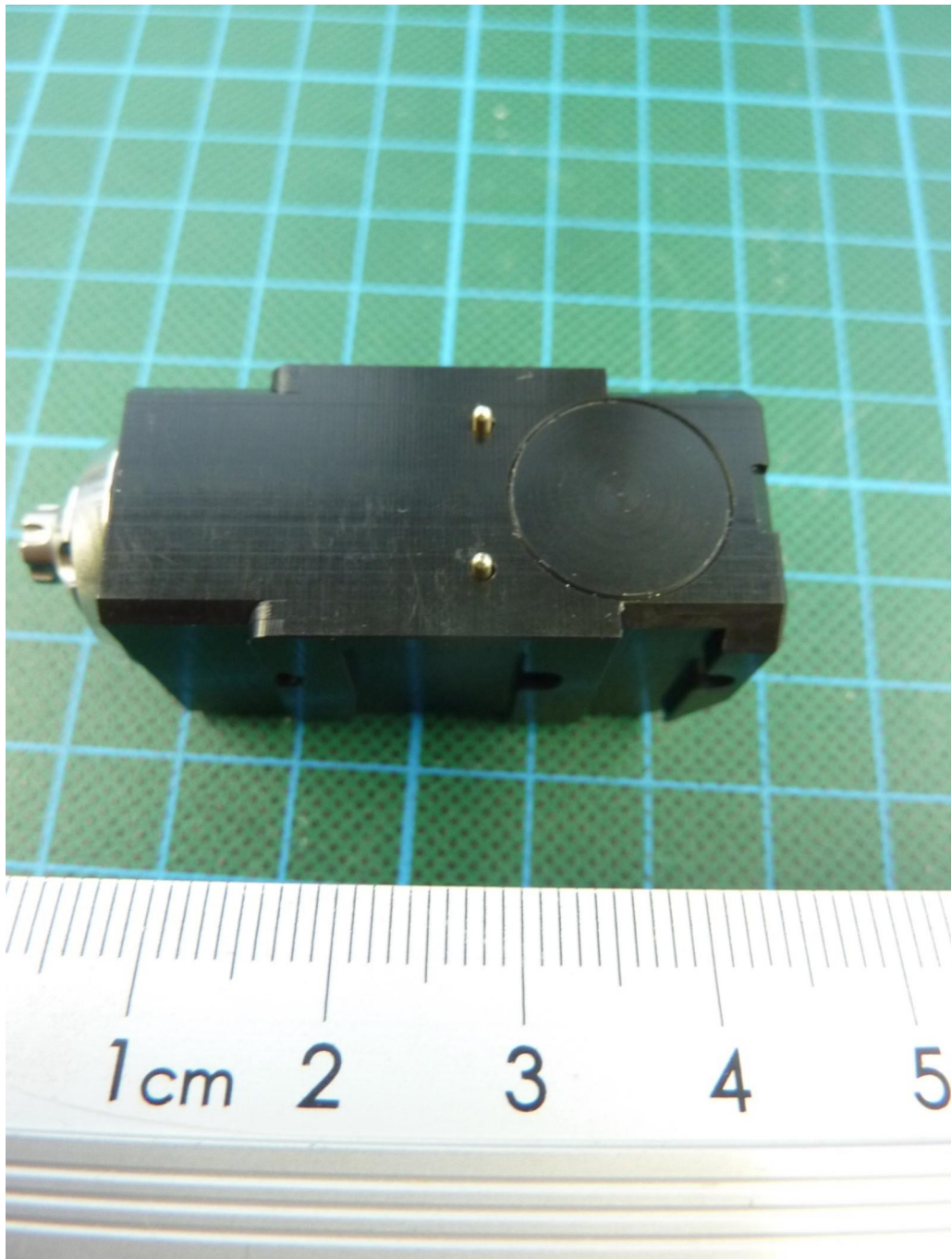
181223_19.jpg: Dosing head QL001 (with TAG), rear view
