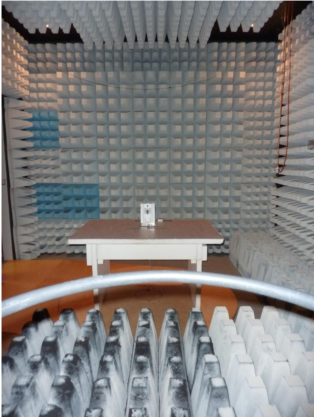
181223_d.jpg: QLX3 liquid module, test setup fully anechoic chamber
