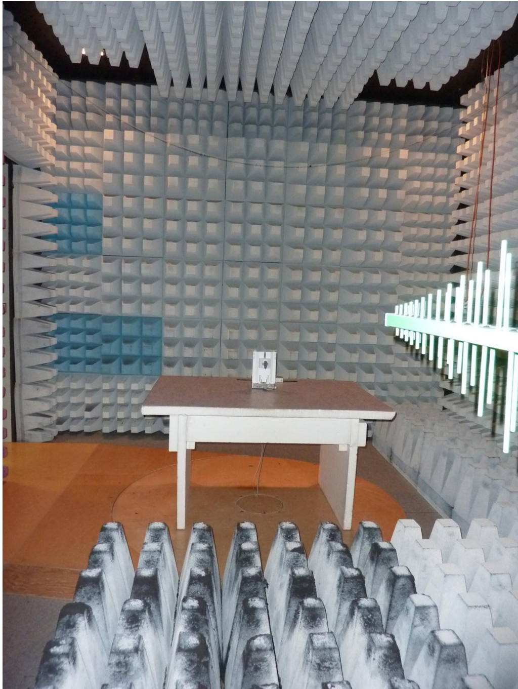
181223_b.jpg: QLX3 liquid module, test setup fully anechoic chamber
