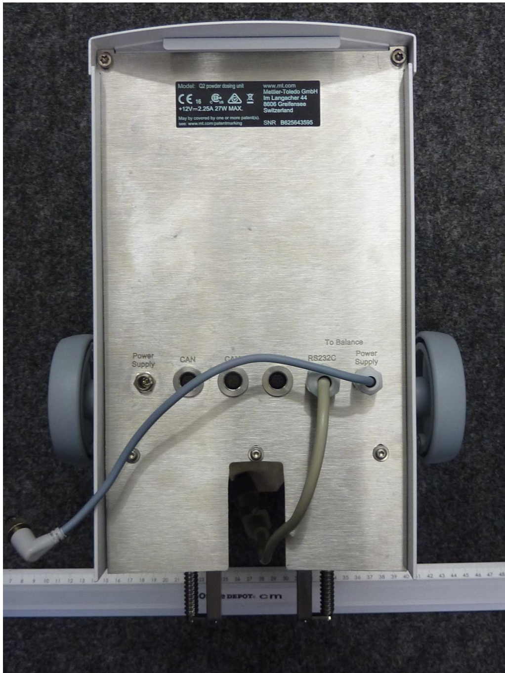
161005_4.jpg: Q2 powder dosing unit, rear view
