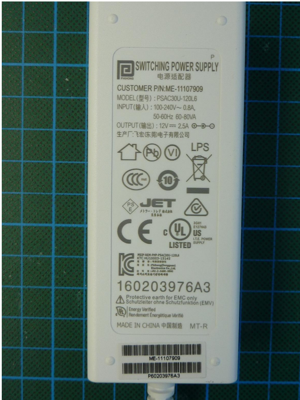
161005_8.jpg: Q2 powder dosing unit, type plate of dedicated AC/DC adaptor
