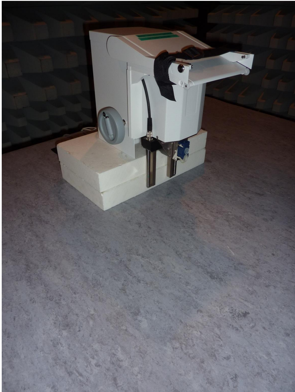
161005_1b.jpg: Q2 powder dosing unit, test setup fully anechoic chamber
