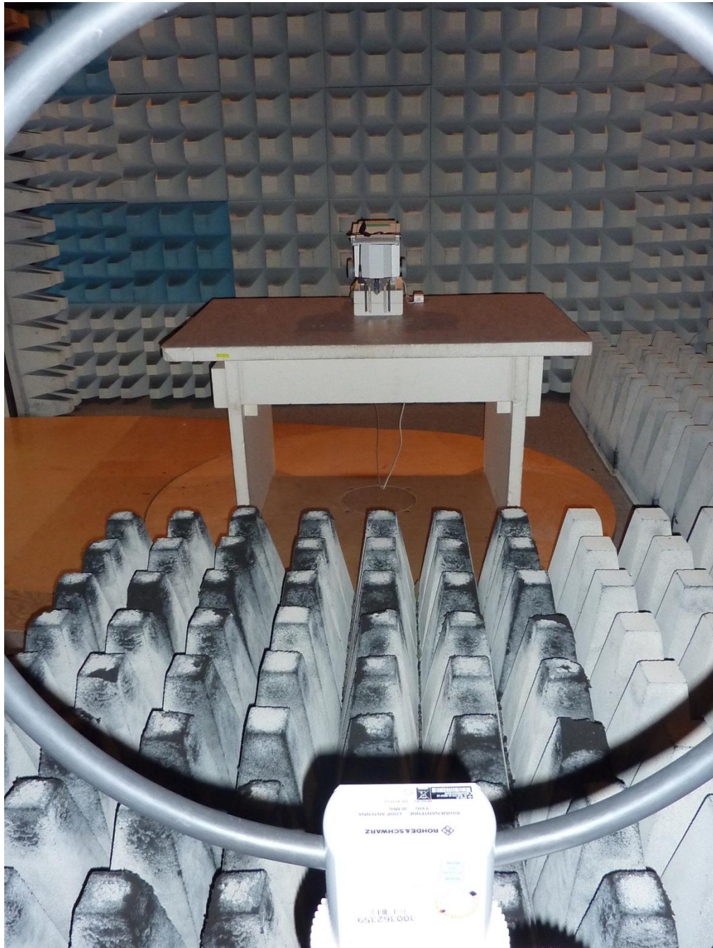
161005_1c.jpg: Q2 powder dosing unit, test setup fully anechoic chamber
