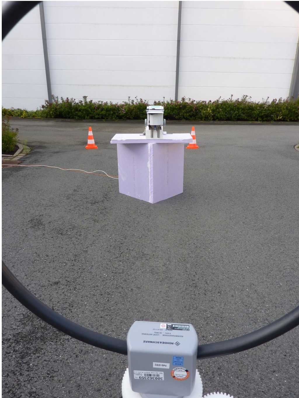
161005_1e.jpg: Q2 powder dosing unit, test setup outdoor test site
