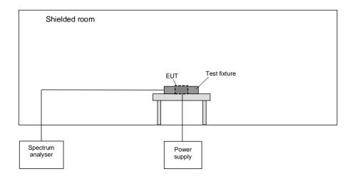
The following procedure will be used for the occupied bandwidth measurement according to [4]:
