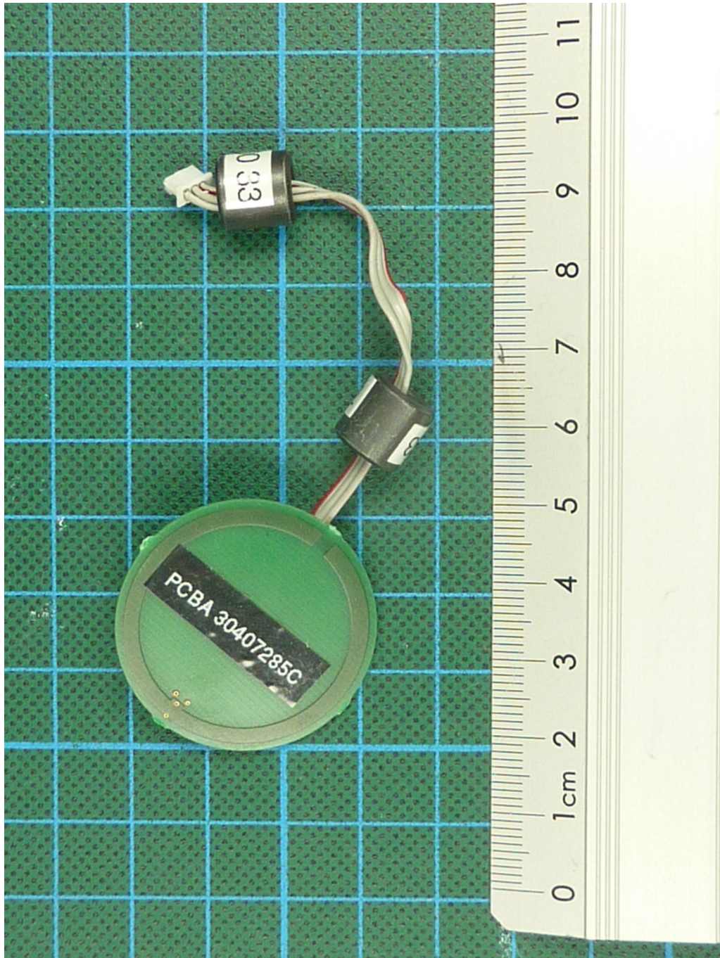
172414_p.jpg: EasyScan USB, 13.56 MHz antenna, top view
