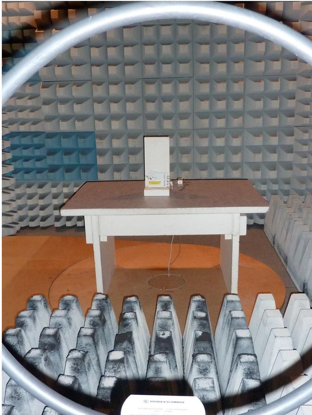
160874_p.jpg: EasyScan Module, test setup fully anechoic chamber
