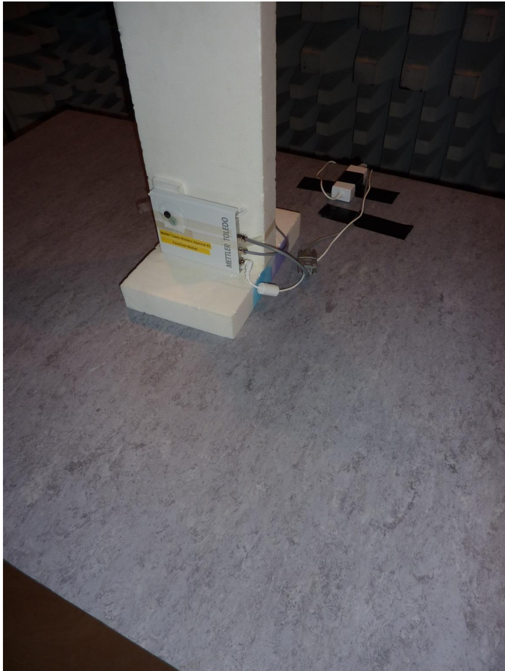
160874_j.jpg: EasyScan Module, test setup fully anechoic chamber
