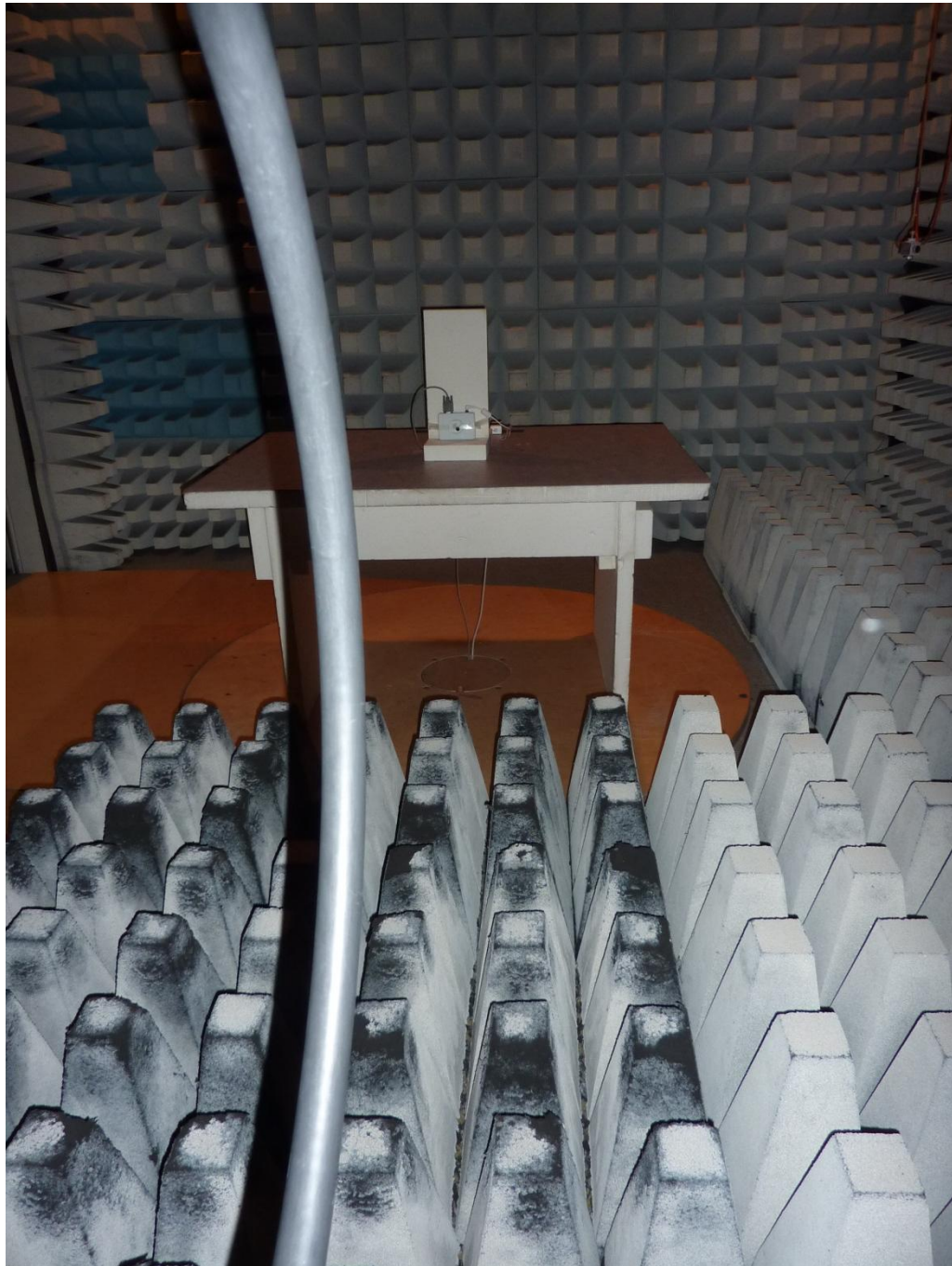
161004_j.jpg: EasyScan Flex, test setup fully anechoic chamber
