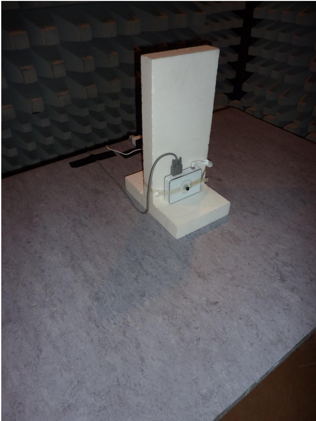
161004_i.jpg: EasyScan Flex, test setup fully anechoic chamber
