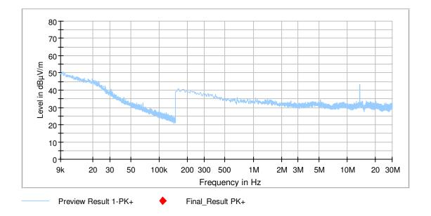
Except the fundamental of the EUT at no frequency was a value above the noise of the system therefore only a final measurement for the fundamental on the open area test site was carried out. No spurious emissions caused by the equipment under test were found.
