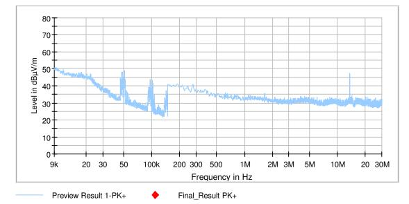
172251Xah1FCCac: Spurious emissions from 9 kHz to 30 MHz (with AC adapter)
