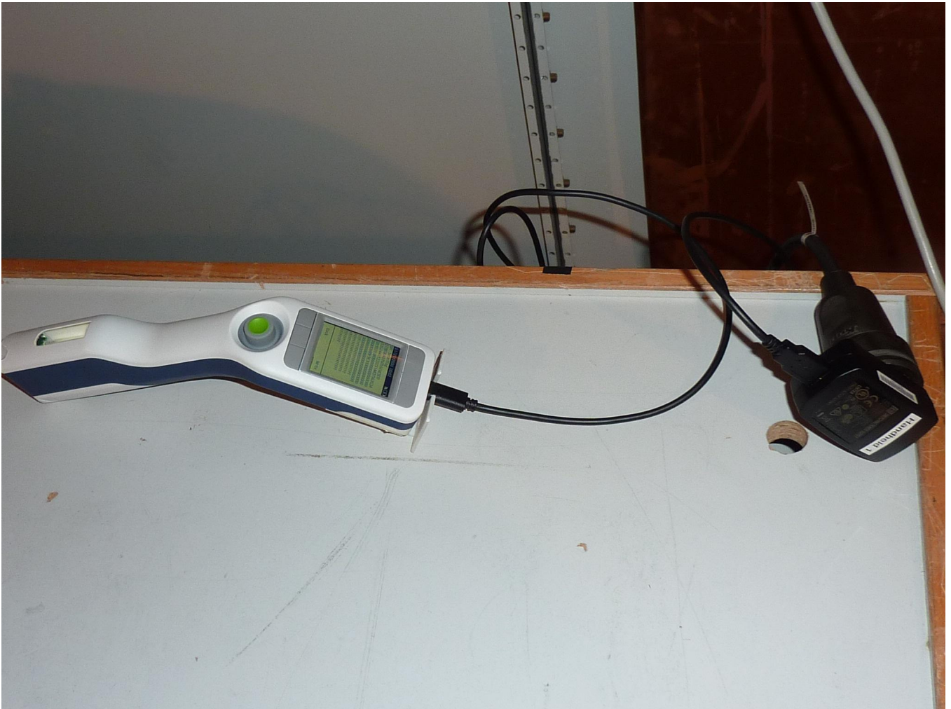
172251_209_01: test setup conducted emission test
