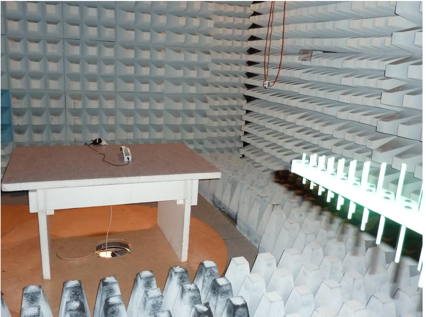
172251_209_05: test setup electric field strength fully anechoic chamber
