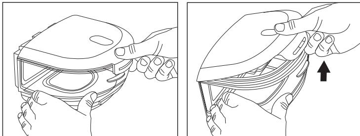
4. Pour out any remaining water and rinse the water tank base.
