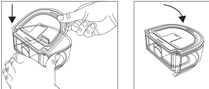
7. Before reinstalling the humidifier water tank, fill it with distilled water no higher than the maximum fill line.
