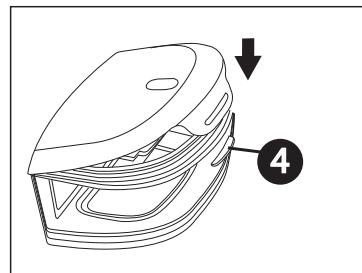
4. Slide the humidifier water tank back into the device, using the tracks on the bottom of the water tank base for proper alignment and connection. Ensure that it is latched into place before proceeding.
