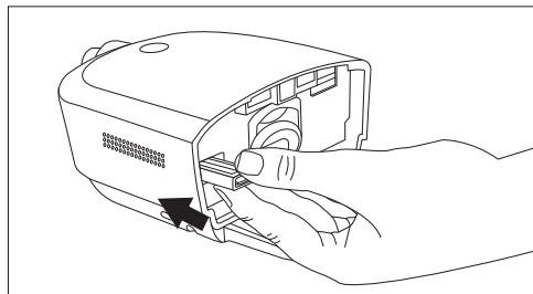
5. Reinstall the humidifier water tank.
