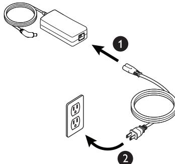
**Important:** To remove AC power, disconnect the power supply cord from the electrical outlet.
