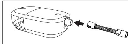
2. Press the heated tubing into place over the air outlet port until the tabs on the side of the tube click into place in the slots on the sides of the outlet port.
