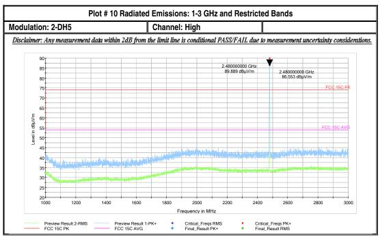
Note: The peak signal above is the Bluetooth transmit signal.
