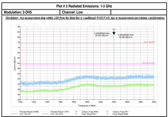
Note: The peak signal above is the Bluetooth transmit signal.
