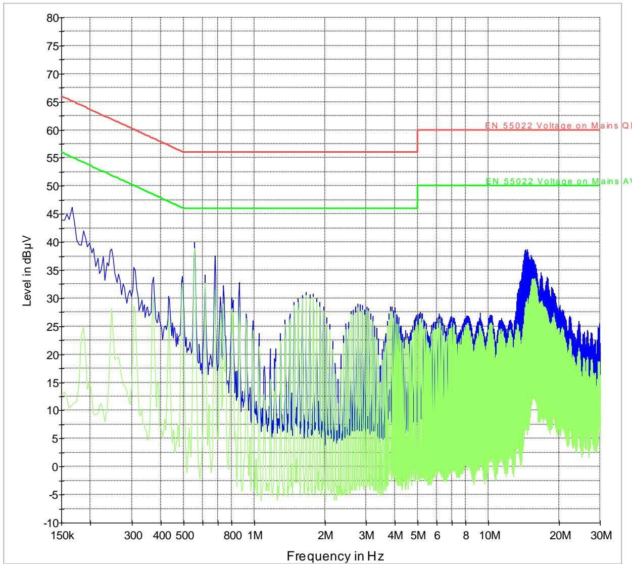
— EN 55022 Voltage on Mains QP.Limit Line EN 55022 Voltage on Mains AV.Limit Line Preview Result 1 Preview Result 2
