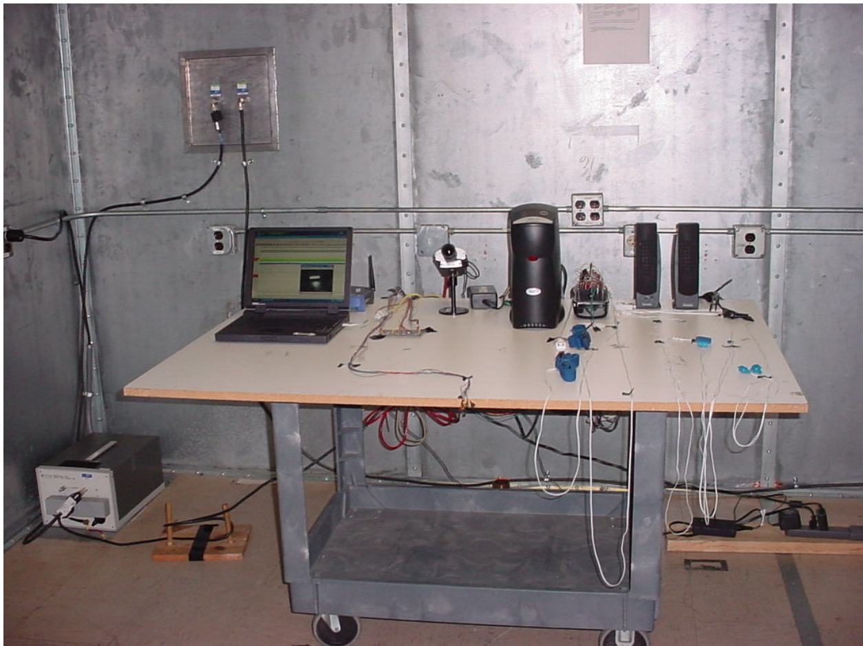
Figure A.1 – Conducted Emissions Test Setup
