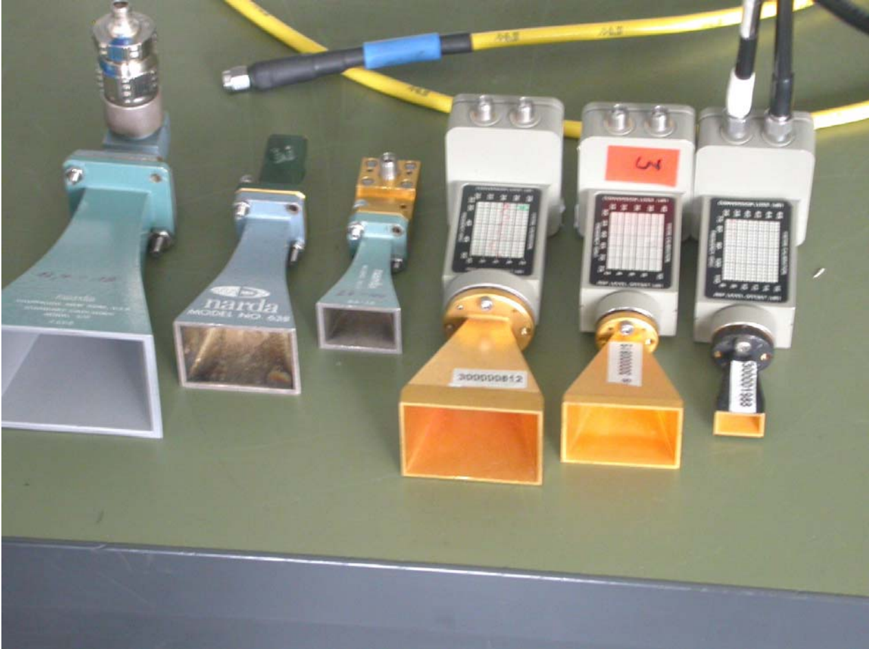
AXR-24 Spurious radiated measurement 12.0 GHz – 100.0 GHz Standard gain horns and Mixer 33.0 GHz – 110.0 GHz
