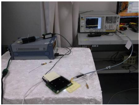
Radiated Emissions Test Configuration Photographs
