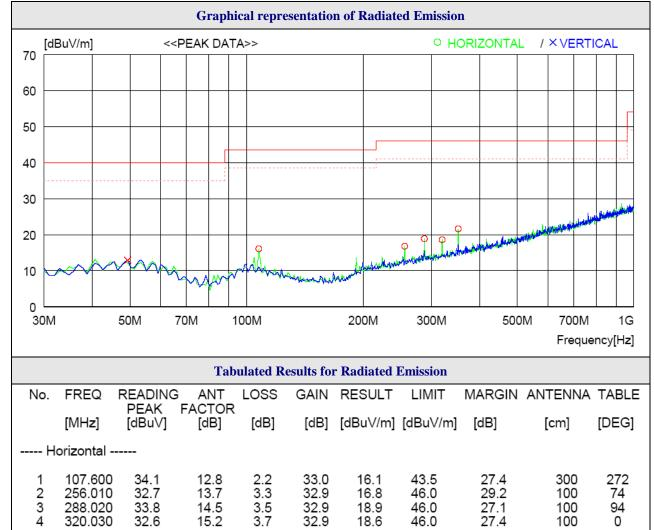
Remark: Margin (dB) = Limit – Result and Result = Reading Peak + Antenna Factor + Loss – Gain Loss and Gain in above table means Cable Loss and Pre-amplifier gain.
