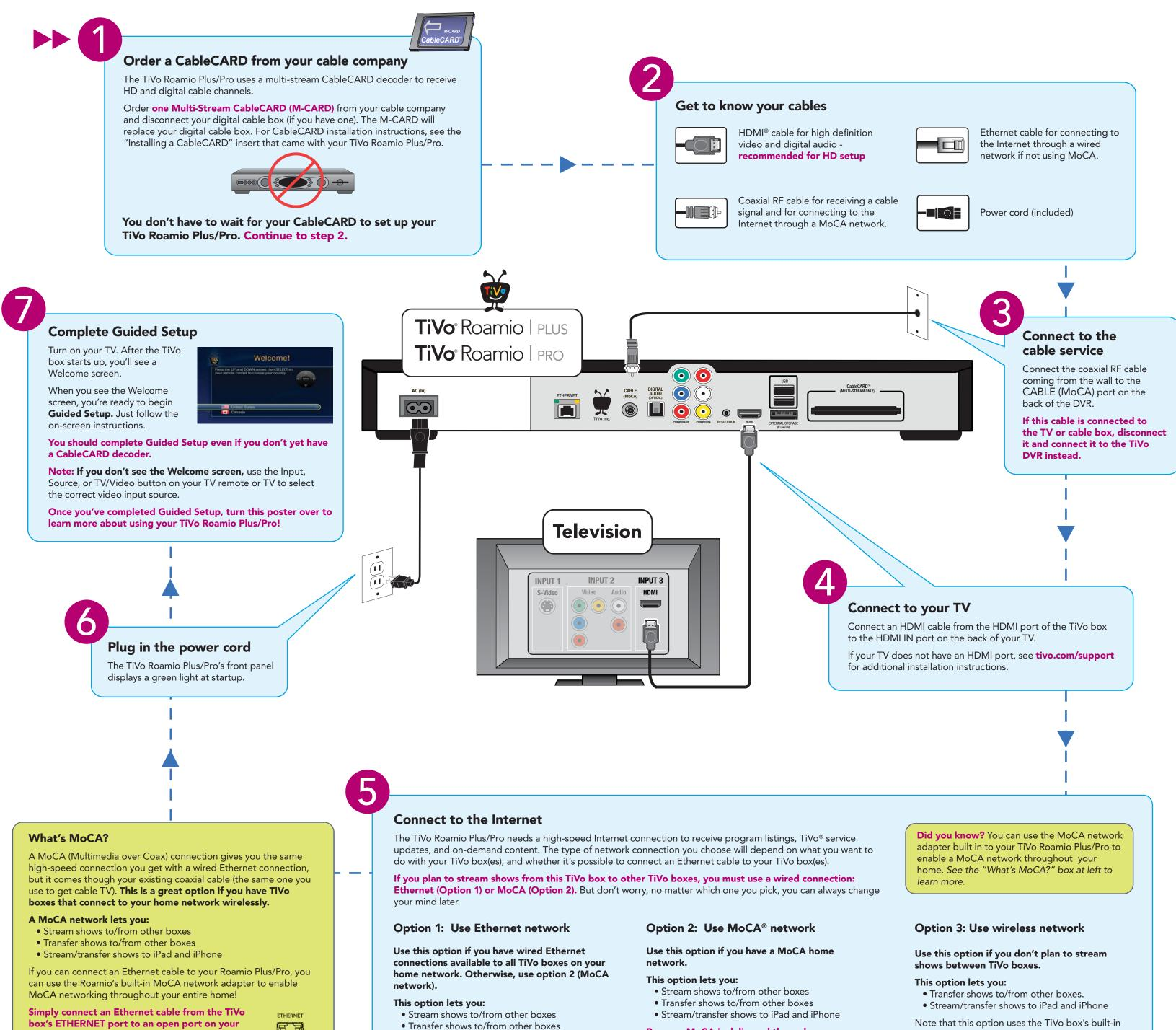
router or to an Ethernet jack in your wall. After Guided Setup, go to Settings > Network > Ð Change Network Settings. Then choose "Use this DVR to create a MoCA network."
