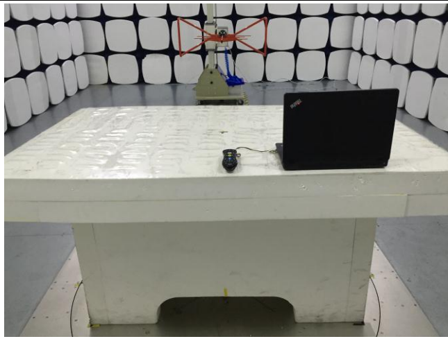
Radiated Spurious Emissions Test Setup Below 1GHz
