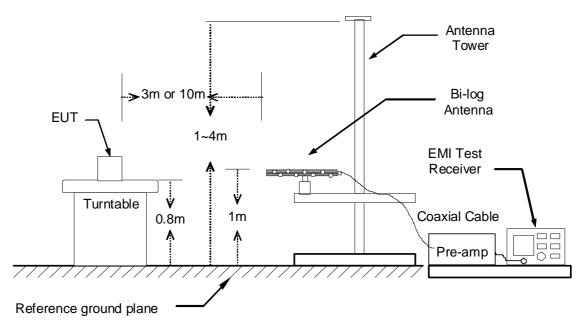
The diagram below shows the test setup that is utilized to make the measurements for emission above 1GHz.
