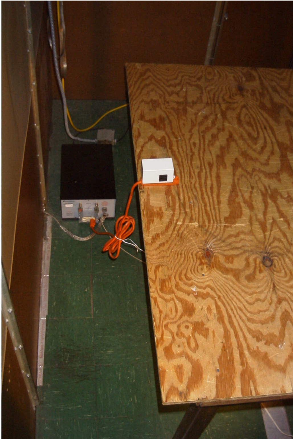
POWERLINE CONDUCTED EMISSIONS TEST SET UP PHOTO
