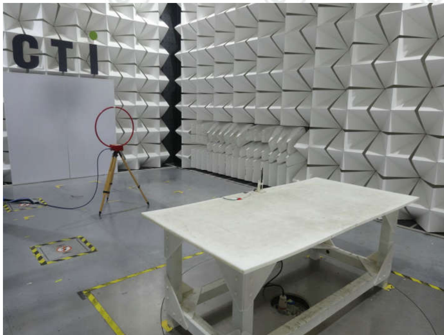
Radiated spurious emission Test Setup-1(Below 30MHz)
