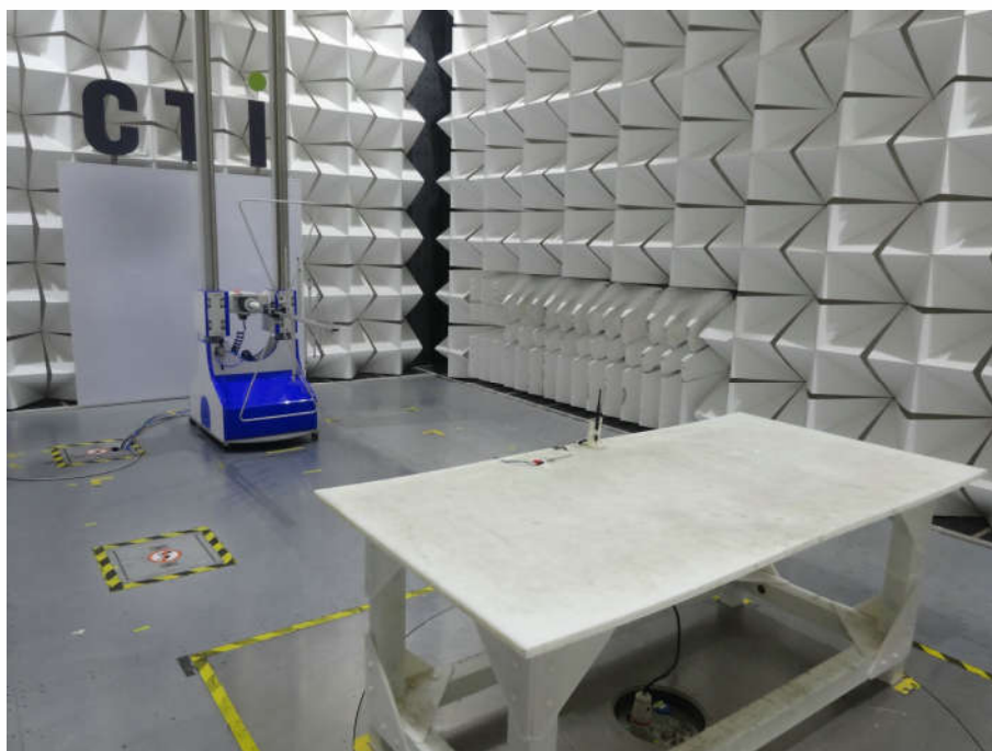
Radiated spurious emission Test Setup-2(30MHz-1GHz)
