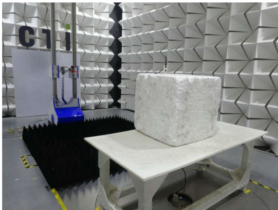
Radiated spurious emission Test Setup-3(Above 1GHz)
