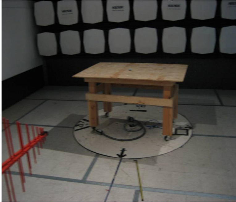
Radiated Emission Test Setup Front View
