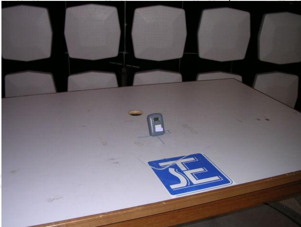
Measurement of Radiated Emission Test Set Up
