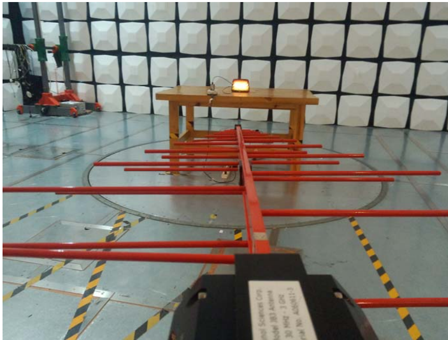
Radiated Emission View (Below 1GHz)
