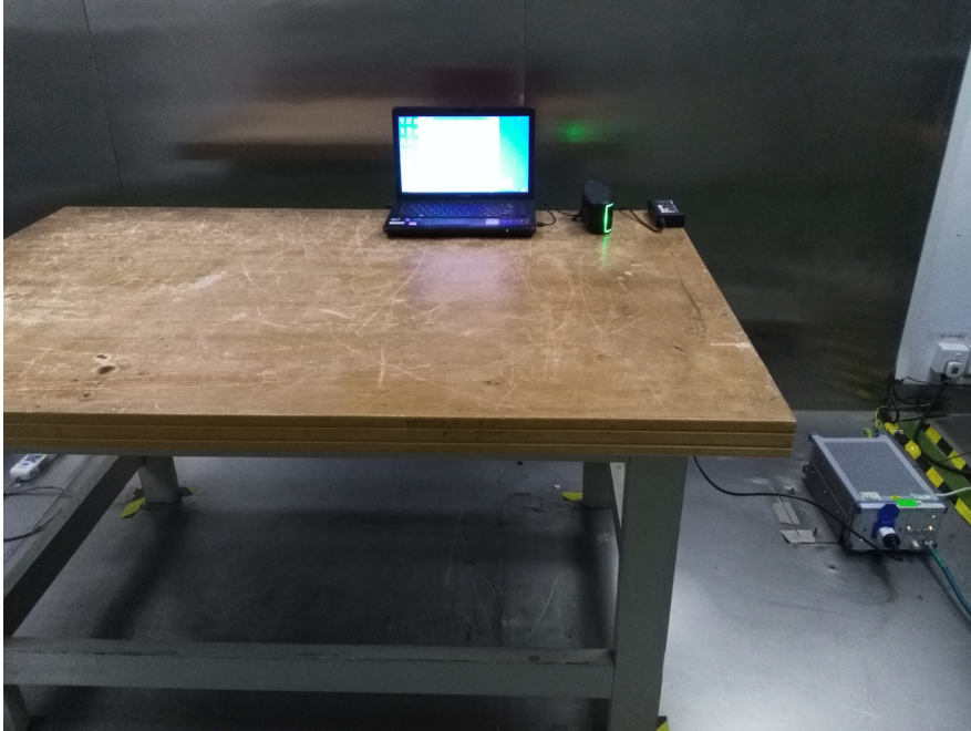
Conducted Emissions - Front View
