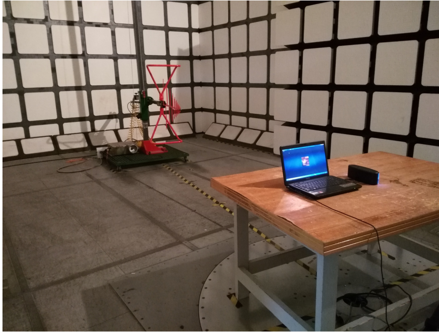
Radiated Emissions View (Below 1 GHz)
