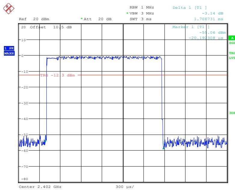
**Pulse time, Middle Channel, 3DH3**
