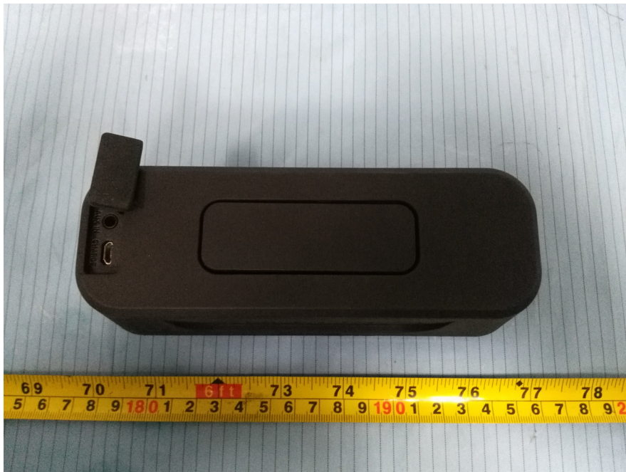
EUT – Audio Port & USB Port View
