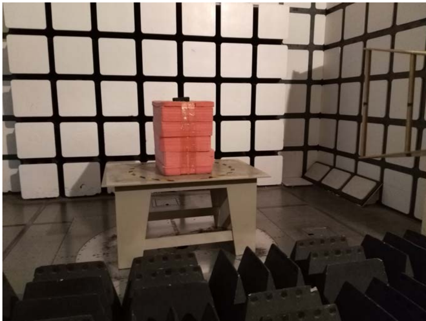
Radiated Emissions View (Above 1 GHz)
